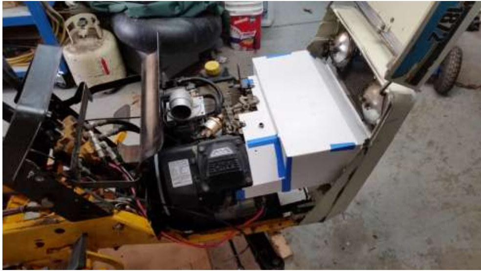
Thin posterboard makes great templates for sheetmetal work.
