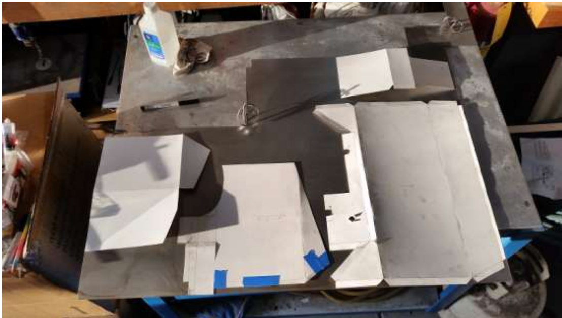
Thin posterboard makes great templates for sheetmetal work.
