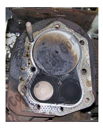
Next, clean the top of the piston, valves, and combustion chamber. I typically use a wire brush, razor blade (take care not to scratch the piston) dental pick, and brake cleaner. If you use brake cleaner, be careful. It's great stuff because it dissolves nearly any type of dirt (including carbon buildup) but it has NASTY fumes and will also wash oil off the rings, so re-oil the piston after using it. This can be seen in the picture below:
