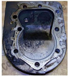
This particular engine didn't have too much carbon buildup, which I've found to be rather unusual. Most engines have so much carbon that I wonder how the engine was operating at all. The failed area of the head gasket is obvious; notice the oil around the exhaust valve area of the head. This is the most common head gasket failure area that I have seen. The spark plug looks pretty good:
