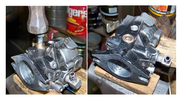
Next, reinstall the throttle shaft and butterfly valve. DO NOT attempt to re-use the brass screws you removed, as they'll just twist off when you try to reinstall them. Don't ask how I know this. Pick up some new screws (I think they're #3-48) and lockwashers, as well as some blue lock-tite. Install the screws with lockwashers and lock-tite.
